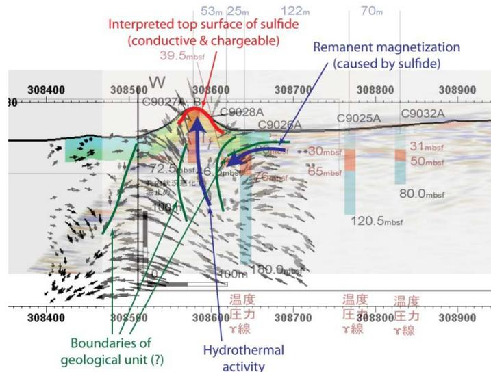
**Figure 7** Vertical cross section of the interpreted structure.
