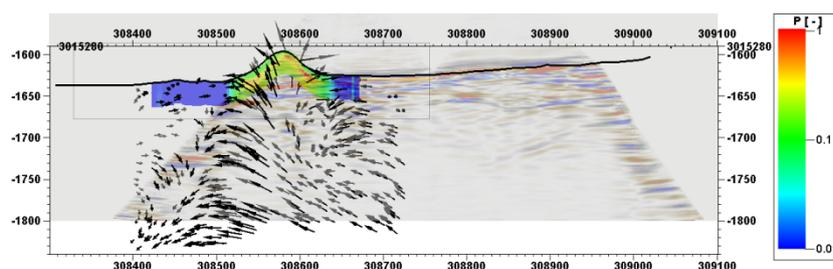
**Figure 6** Vertical cross section of 3D chargeability and 3D magnetization vector models recovered by the guided 3D inversions overlaid with seismic data.
