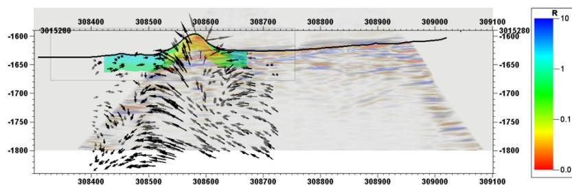
**Figure 5** Vertical cross section of 3D resistivity and 3D magnetization vector models recovered by the guided 3D inversions overlaid with seismic data.
